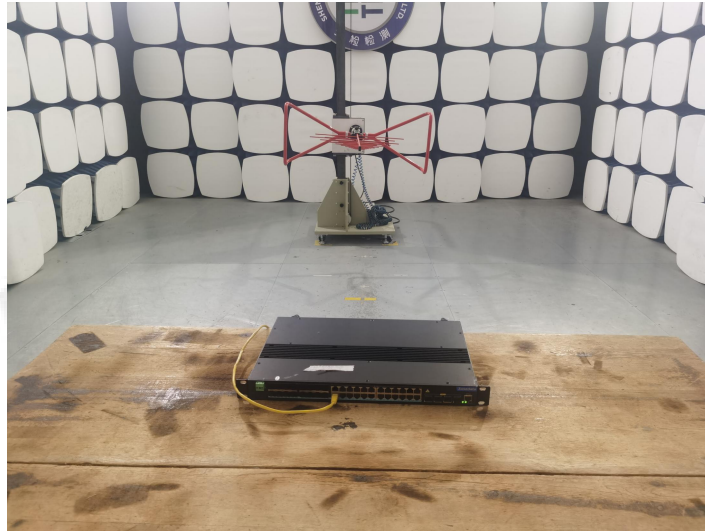
RADIATED EMISSION TEST(Above 1000MHz)
